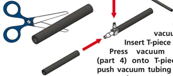
Cut into vacuum pipe. Insert T-piece (part 7). Press vacuum damper (part 4) onto T-piece then push vacuum tubing (part 3) into vacuum damper.
