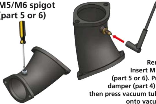
Remove screw. Insert M5/M6 spigot (part 5 or 6). Press vacuum damper (part 4) onto spigot then press vacuum tubing (part 3) onto vacuum damper.
