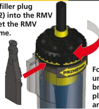
Connect spout to the filler plug and squeeze bottle.
