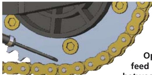
Optimum feed point is between 5 & 7 o'clock on the face of the rear sprocket.
