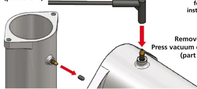
Remove bung. Press vacuum damper (part 4) onto spigot.
