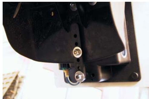
Using the 10mm spacer in the HCR kit, bolt the HCR Adapter bracket to the HCR as shown above. If you have any queries or comments, or require any additional parts, please don't hesitate to contact our technical department.
