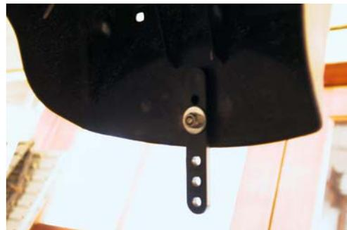
Fit the bracket to the mudguard using the middle hole on the bracket, and the bolt and washers as shown in the above photographs.
