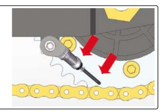
4. Route the delivery tubing from the dispenser back toward the reservoir by routing the delivery tubing inside the swing arm to behind the rear suspension unit and up towards the reservoir on the subframe.
