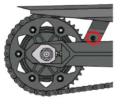
1. Remove the rear chain guard mounting bolt using a T30 Torx wrench, it is not necessary to remove the chain guard itself.
