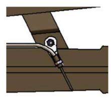
3. Secure the Dispenser Assembly (part 14) to the Dispenser Plate (part 16) by clamping around the black nylon sleeve using the Dispenser Plate Clip (part 17).
